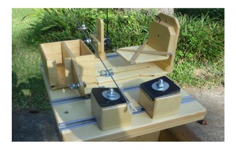
THIS IS THE SET-UP FOR RUNNING A BEAM MOUNTED ENGINE GLOW OR GASOLINE. USE THE BATTERY BOX TO HOLD THE IGNITION MODULE.
