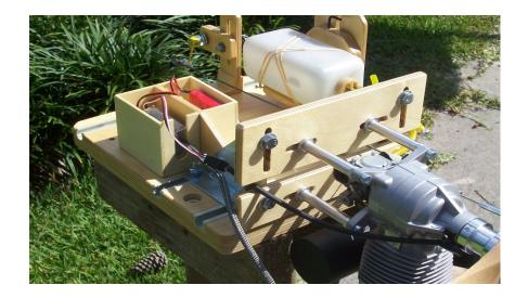
THIS IS THE SET-UP FOR RUNNING RADIAL MOUNTED ENGINES USING STAND-OFFS. THE BATTERY BOX ALSO HOLDS THE IGNITION MODULE.
