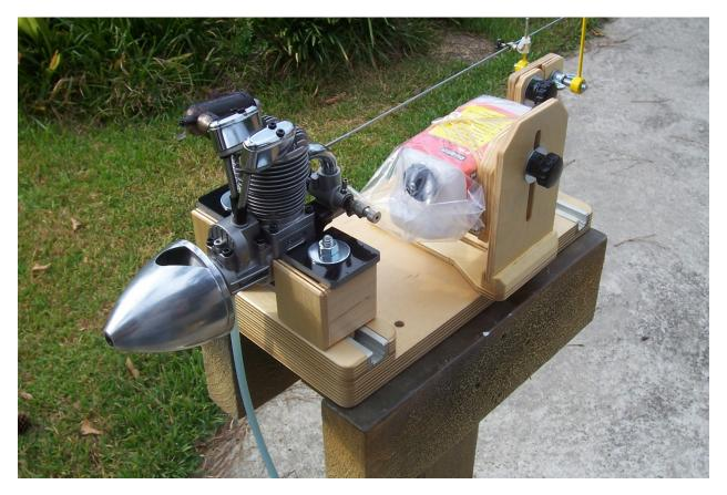
THE "SMALL STAND" WAS DESIGNED TO HOLD 2 AND 4 CYCLE ENGINES THAT HAVE BEAM MOUNTING. IT WILL HOLD LARGE ENGINES TO 2.0 CU. IN. YOU CAN ALSO RUN THE SMALL GASOLINE ENGINES, BUT I SUGGEST THE LARGE STAND AS IT HAS A BOX TO HOLD THE IGNITION MODULE AND BATTERY.
